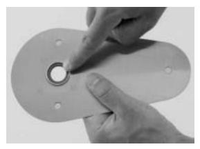
With the convex side of the shaft seal facing up (and the concave, ridge side facing down), snap the new shaft seal onto the bin insulator plate.
